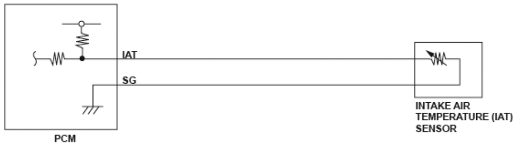
Fig. 8: Intake Air Temperature (IAT) Sensor Circuit Diagram
