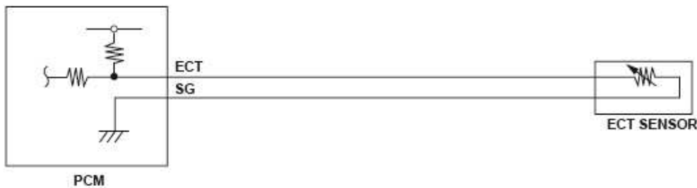
Fig. 15: Engine Coolant Temperature (ECT) Sensor Circuit Diagram
