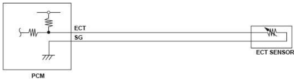
Fig. 13: Engine Coolant Temperature (ECT) Sensor Circuit Diagram
