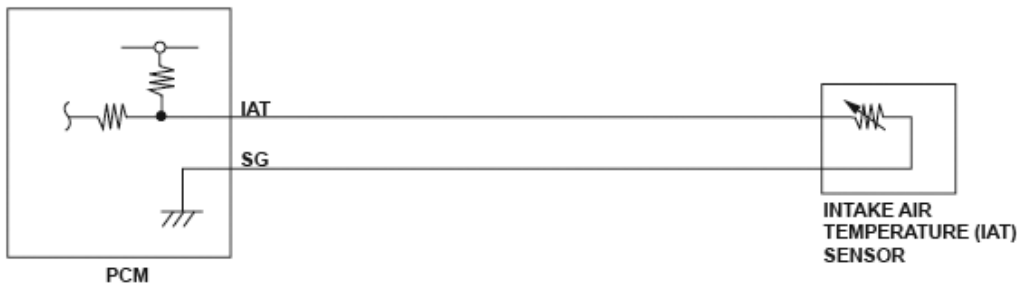
Fig. 10: Intake Air Temperature (IAT) Sensor Circuit Diagram
