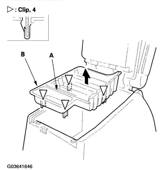
Fig. 1: Pulling CD Storage Box Courtesy of AMERICAN HONDA MOTOR CO., INC.
