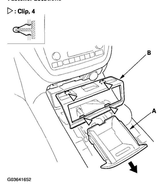
Fig. 7: Removing Coin Pocket Courtesy of AMERICAN HONDA MOTOR CO., INC.
