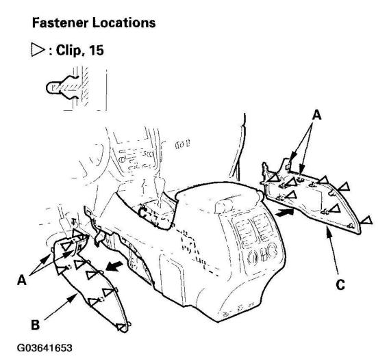
Fig. 8: Detaching Clips And Release Hooks Courtesy of AMERICAN HONDA MOTOR CO., INC.
