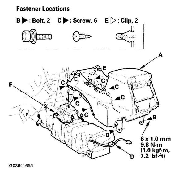
Fig. 10: Removing Center Console Courtesy of AMERICAN HONDA MOTOR CO., INC.
