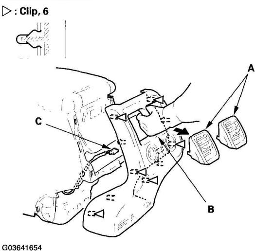
Fig. 9: Removing Vents Courtesy of AMERICAN HONDA MOTOR CO., INC.
