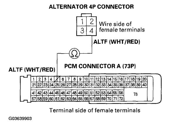
Fig. 5: Checking Continuity Between Alternator 4P Connector Terminal No. 4 And PCM Connector Terminal A25 Courtesy of AMERICAN HONDA MOTOR CO., INC.
