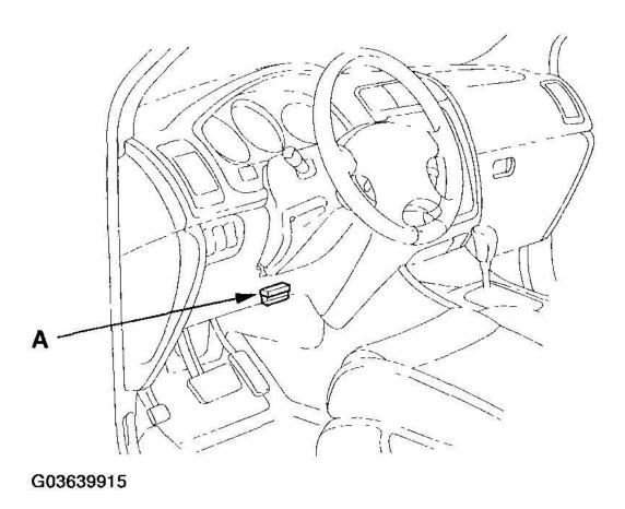
Fig. 17: Connecting HDS To DLC Courtesy of AMERICAN HONDA MOTOR CO., INC.
