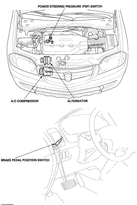
2003-06 ENGINE PERFORMANCE Idle Control System - MDX
