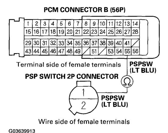
Fig. 15: Checking Continuity Between PCM Connector Terminal B55 And PSP Switch 2P Connector Terminal No. 1
