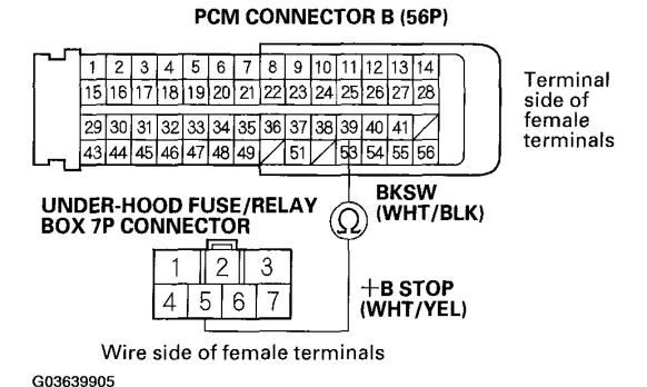
Fig. 7: Checking Continuity Between PCM Connector Terminal B39 And Under-Hood Fuse/Relay Box 7P Connector Terminal No. 5
