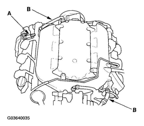
Fig. 1: Checking PCV Valve, Hoses, And Connections For Leaks Or Restrictions Courtesy of AMERICAN HONDA MOTOR CO., INC.
