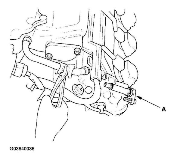
Fig. 2: Pinching PCV Valve Courtesy of AMERICAN HONDA MOTOR CO., INC.
