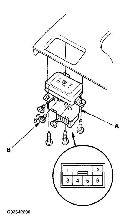
Fig. 7: Disconnecting 6P Connector From Seat Heater Switch Courtesy of AMERICAN HONDA MOTOR CO., INC.
