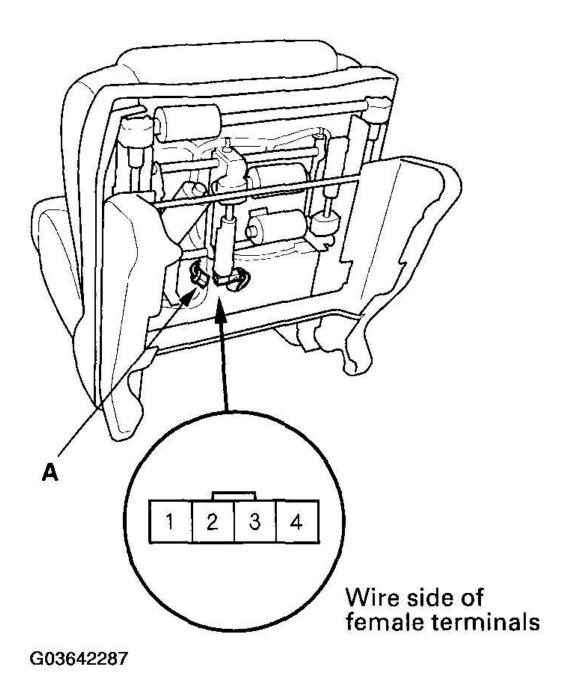
Fig. 4: Disconnecting 4P Connector From Seat Heater Courtesy of AMERICAN HONDA MOTOR CO., INC.
